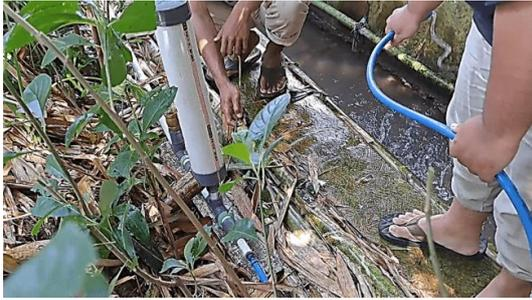
Gambar 6. Pengecekan *output* pompa hydrum
