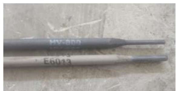
Gambar 3.1 Elektroda HV-800 – 4 mm × 350 mm, (B).Elektroda E6013 – 4 mm × 350 mm
